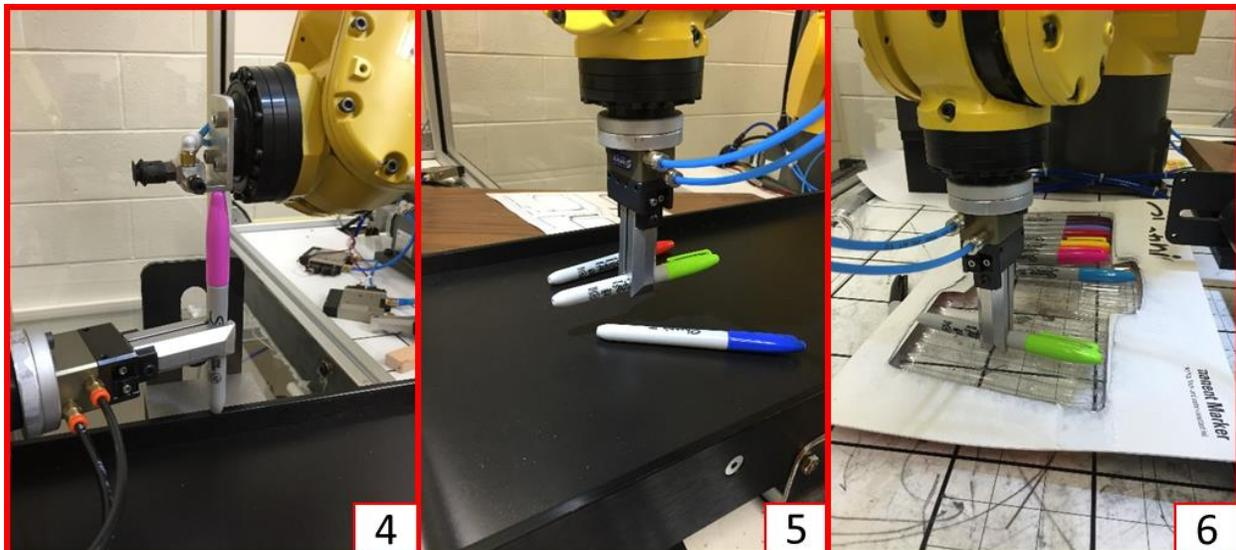
Figure 11. 4) Robot 3 tightens the cap by pressing it on the marker 5) Robot 1 picks the assembled marker 6) Robot 1 places the assembled marker on the tray
