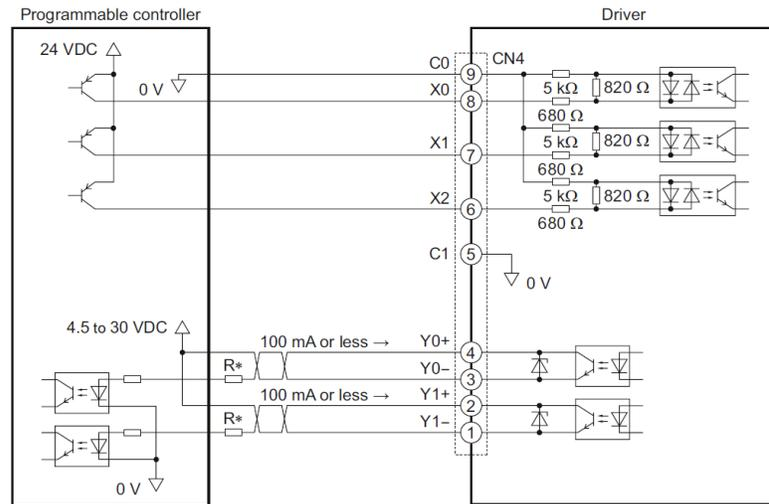
Figure 5. Connection from PLC to the VFD using source logic
