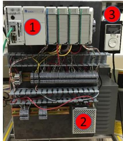
Figure 4. 1) Programmable Logic Controller, 1769-L32E 2) Switch Mode Power Supply, S82J-0224 3) Variable Frequency Drive, BMUD60-A2
