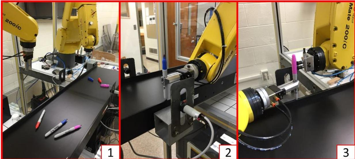
Figure 10. 1) Initial setup with open markers and caps 2) Robot 2 picks the open marker and places it for assembly 3) Robot 3 assembles the cap on the marker
