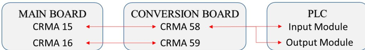
Figure 6. Wiring Connections between the PLC and Robot Controller
