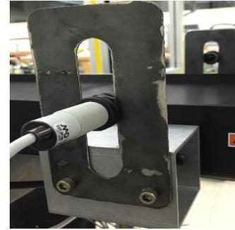
Figure 2. Through beam sensor mounted on brackets
