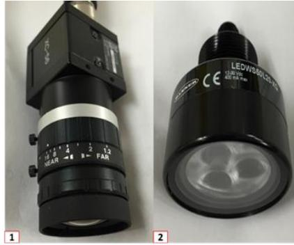
Figure 3. 1) XC-56 Sony Camera 2) LED spot light
