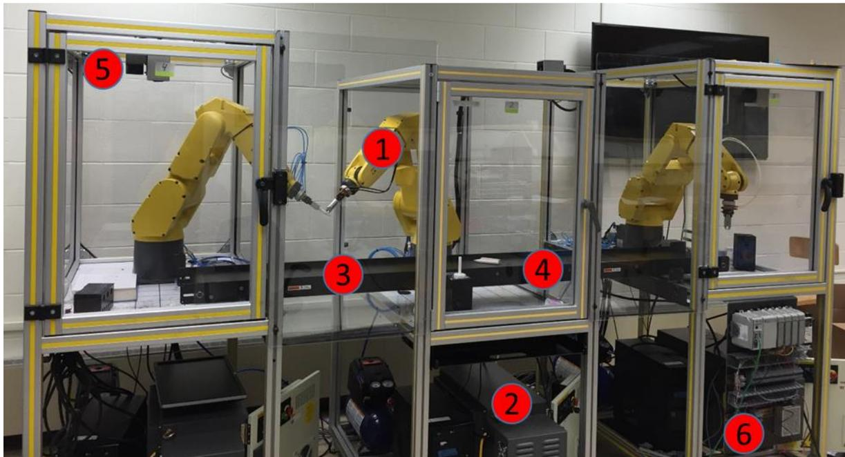
Figure 1. The work cell consisting of 1) Robot 2) Robot Controller 3) Conveyor 4) Sensors 5) Vision system 6) Control Panel
