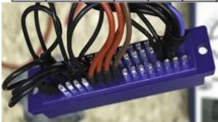
Where, Pin no. 1-16 represent DI101-DI116 (Digital inputs)
