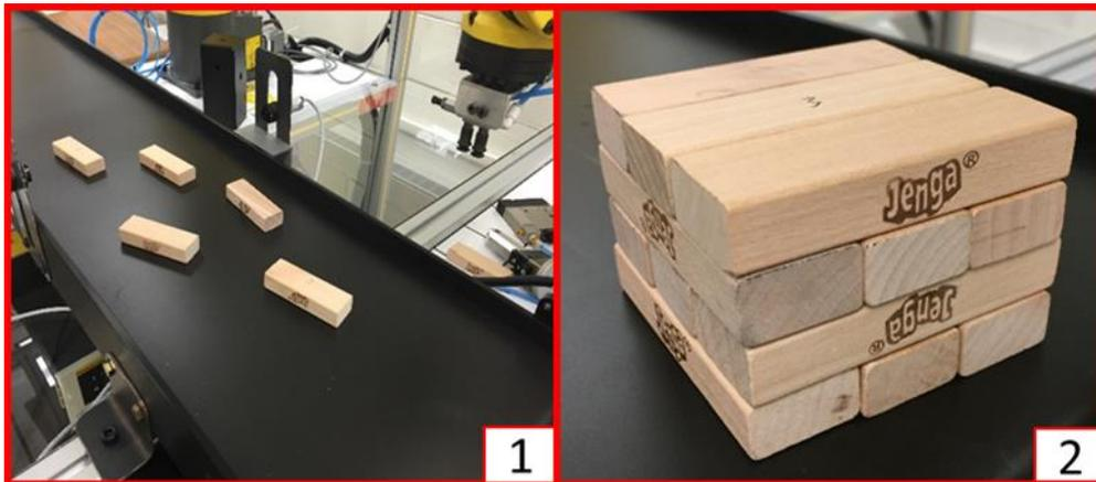
Figure 9. 1) Randomly placed Jenga blocks travelling on conveyor 2) Final Pallet formed by the robot
