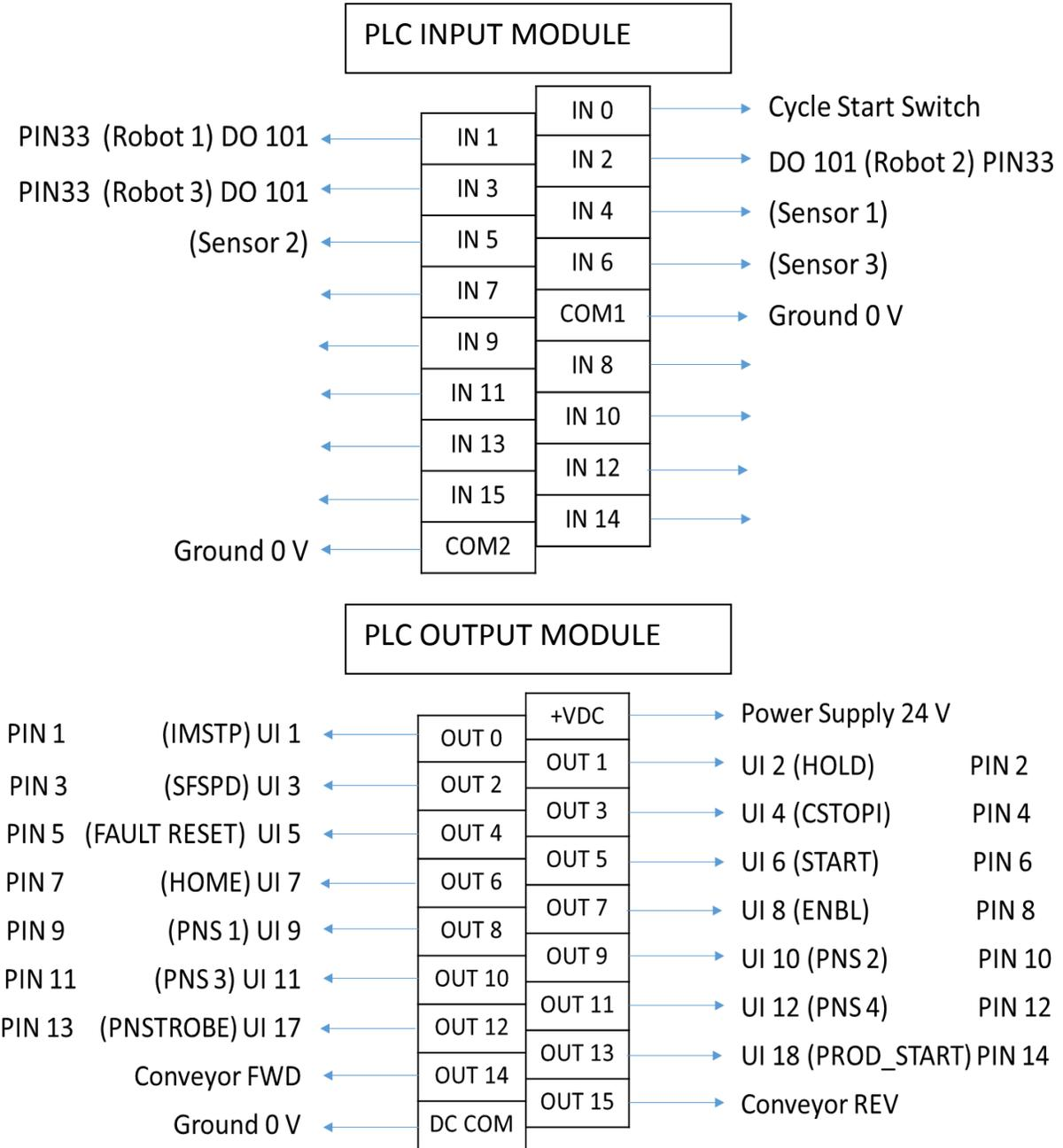
Figure 8. PLC I/O to UI/UO connections
