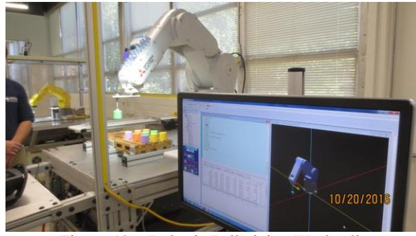
Figure 13 – Robotic Palletizing Workcell
