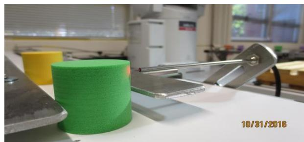
Figure 10 – I/O sensors on the conveyor
