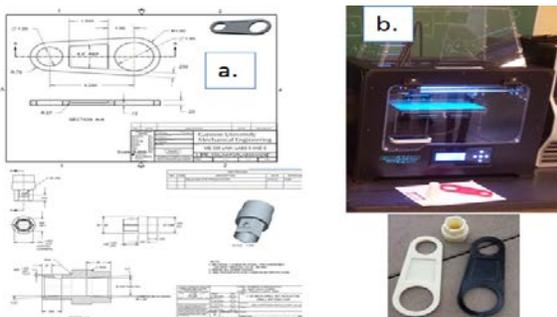
**Figure 5:** Lab 5, 3D Printing, a) link and drill bit end cap, b) one of the FDM printers used for rapid prototyping with samples shown.
