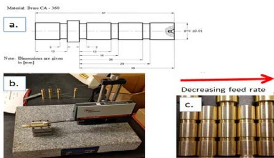
**Figure 3:** Lab 2, Process Capability Study for Surface Finish, a) specimen geometry, b) measuring average roughness, Ra, c) specimens machined at varying feed rate.
