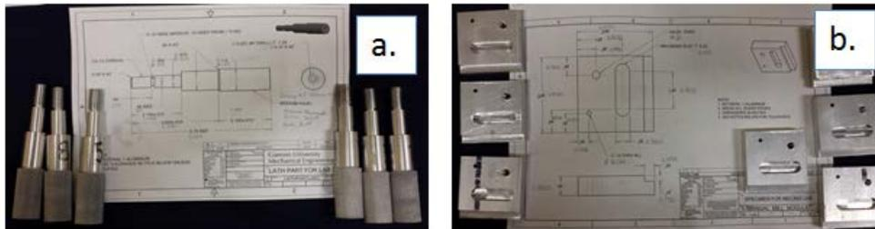
**Figure 4:** Lab 3 and 6, Fundamentals of Machining, a) lathe part, b) mill part. Students are required to machine both parts to spec.
