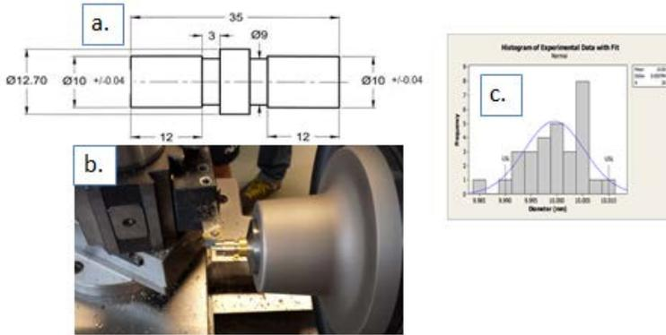
**Figure 2:** Lab 1, Process Capability, a) specimen geometry, b) specimen turning on lathe, c) sample student output from report.
