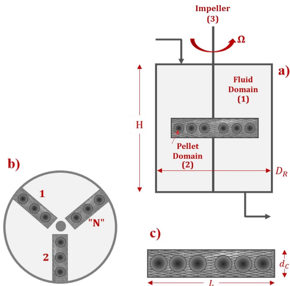
**Figure 1:** “Cilindro Rotador” Sketch: A) The side view of the tank B) The top view showing “N” cylinders on the rotating axis C) The mesh of the cylinder holding the catalytic pellets
