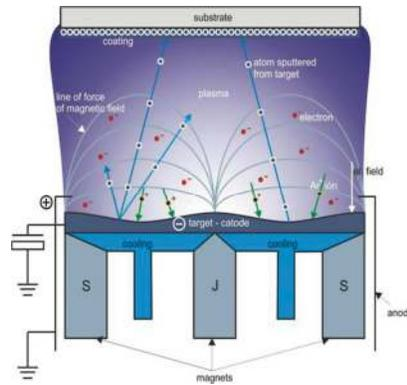
**Figure 4: Sputtering Process<sup>17</sup>**
