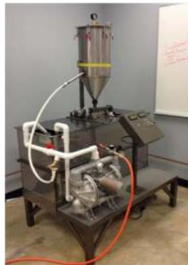
**Figure 2: Erosion Test Fixture**
