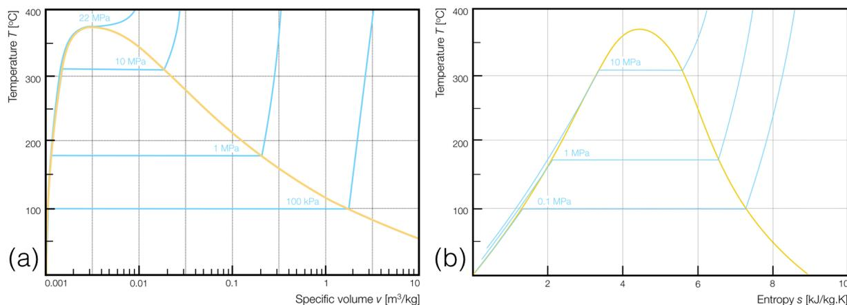
**Figure 2.** (a)  $T$ - $v$  diagram depicting isobars used to demonstrate phase change of water from atmospheric conditions and (b)  $T$ - $s$  diagram with the same isobars to highlight the similarities between the two diagrams and introduce entropy  $s$  as a ‘yet another thermodynamic property’.
