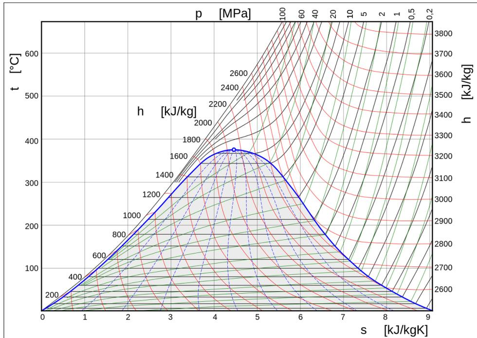
**Figure 1.** A Temperature-Entropy ( $T$ - $s$ ) diagram with red constant enthalpy  $h$  lines, green constant density  $\rho$  lines, and black constant pressure  $P$  lines (isobars). Note: the figure uses  $t$  instead of  $T$  for temperature. Created by *Kaboldy* for *Wikipedia.org*.
