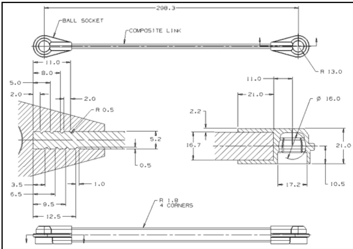
Figure 2 Connecting rod drawing [dong et al, 2016]
