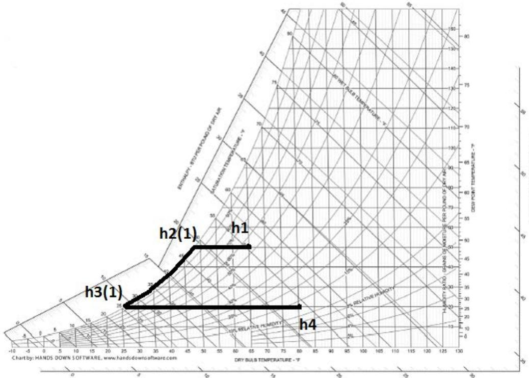
Figure 1: Psychrometric chart plotting the process of method 1
