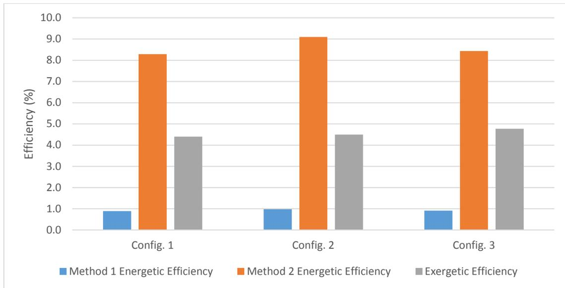
Figure 3: Energetic vs. Exergetic efficiencies for EHD drying.
