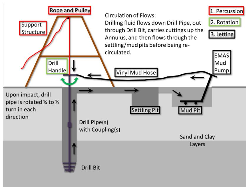
Figure 1. Diagram of the EMAS standard drilling method<sup>1</sup>.
