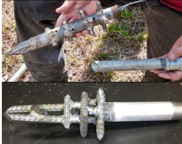
*Figure 3.* Drill bits utilized in this research (from top to bottom): Christmas tree, sand, and universal.
