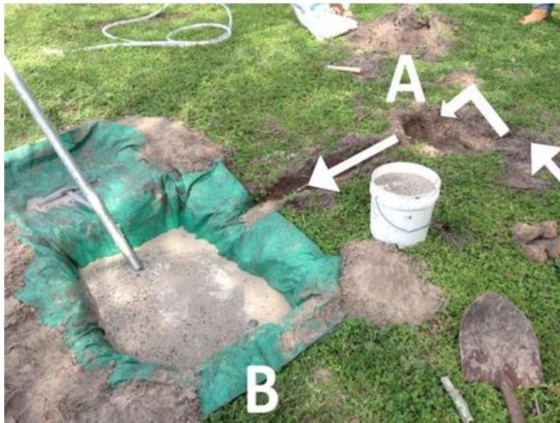
*Figure 4.* Trench pit system, consisting of (A) the settling pit, (B) the mud pit, and connecting trenches dug perpendicular to each other.
