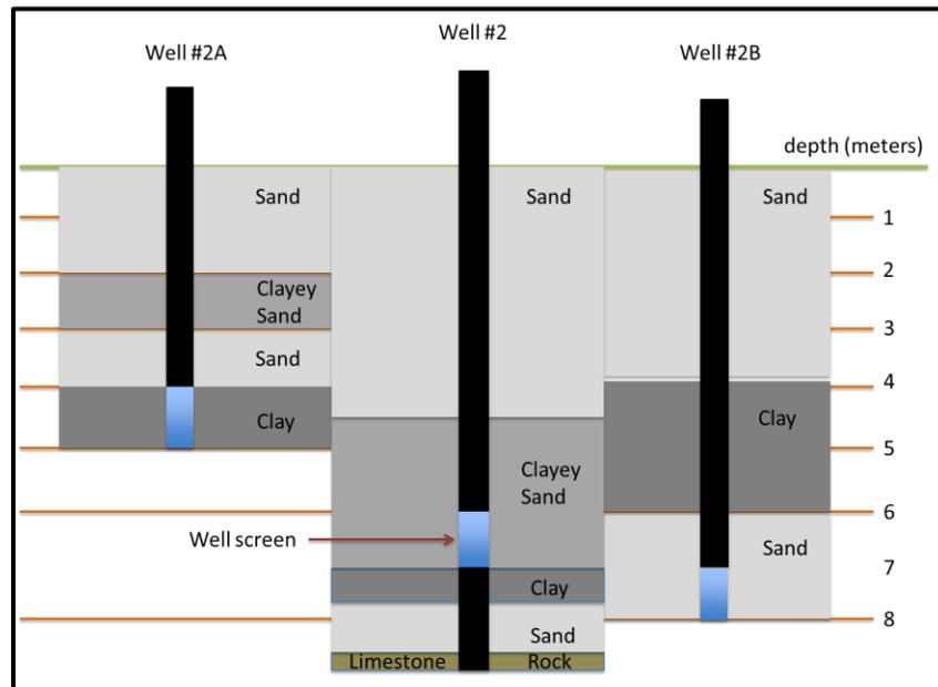
Figure 5. The soil profile for the three wells at Site #2.
