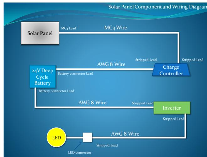
Figure 15: Solar Panel Component Wiring Diagram
