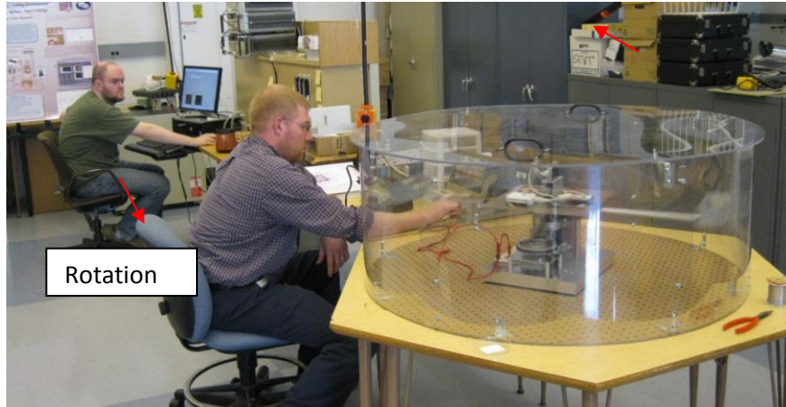
Figure 5. Acceleration Sensor Test Platform under operation
