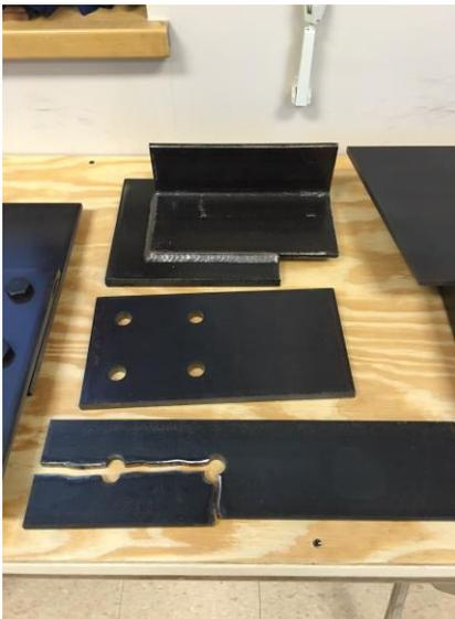
Figure 2: Block Shear & Bolted/Welded Connection Models
