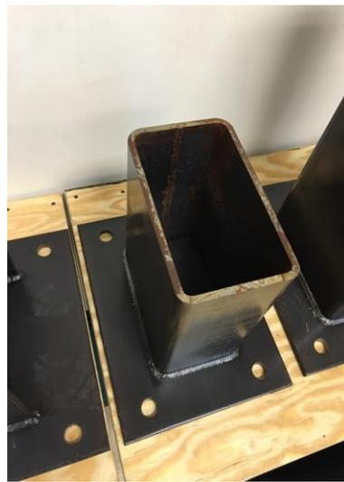
Figure 6: HSS Column and Baseplate Model
