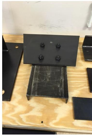
Figure 4: Bolted Channel-Plate Model
