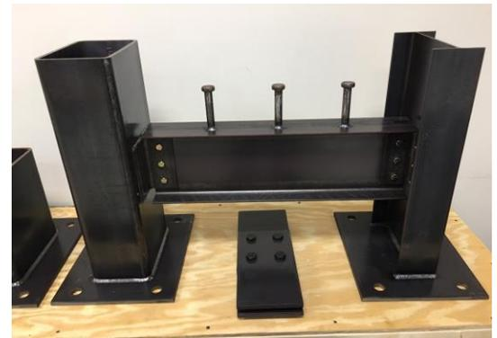
Figure 7: Composite Beam and Bolted Connection Model
