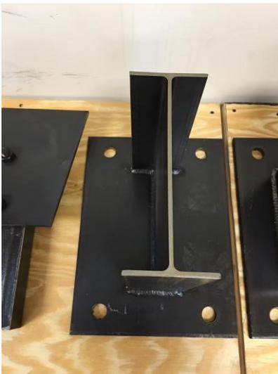
Figure 5: WF Column and Baseplate Model
