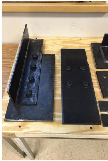
Figure 3: Bolted Angle-Plate and Plate-Plate Connection Models
