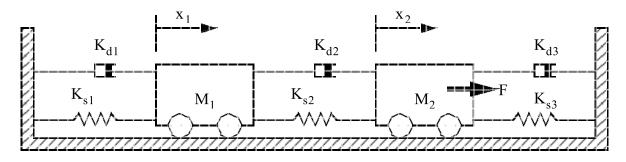
Figure 4- Two degree of freedom mechanical system-Example 2<sup>[4]</sup>
