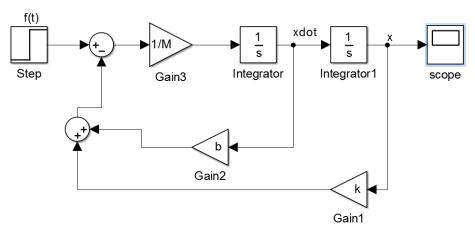
Figure 2- Simulink Model for System in Example 1
