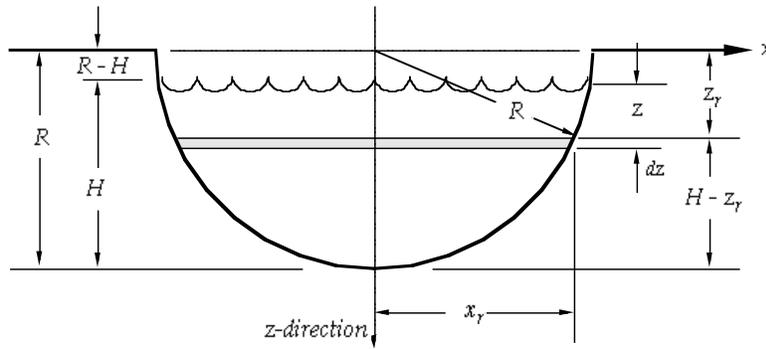
**Figure 1.** Cross section of a semi circular weir.
