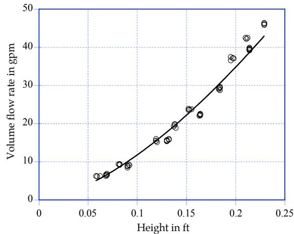
Figure 3. Data points; flow rate over a semi circular weir as a function of upstream water height.
