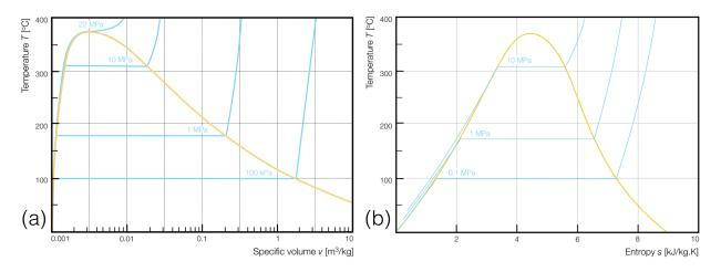
**Figure 2.** (a) T-v diagram depicting isobars used to demonstrate phase change of water from atmospheric conditions and (b) T-s diagram with the same isobars to highlight the similarities between the two diagrams and introduce entropy s as a 'yet another thermodynamic property'.
