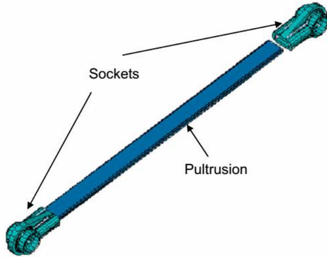
Figure 1 Connecting rod assembly
